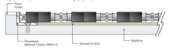
Commence installation with an unshaped mat panel wherever possible, being sure to follow the location indicated in the "Matting order confirmation form". Further panels should then be fitted, ensuring all panels are tight to the divider bars and with no gaps, except for a 1mm tolerance. When fitted correctly, the adjacent panels either side of the divider bars should align.
