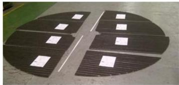
Mats produced to a drawing or template are supplied to a finished size, as requested, and indicated on the "Matting order confirmation form" and should require minimal site adjustment. The mats should then be laid so that the pedestrians walk across the mat ribs, direction of traffic (DOT), and not along them.
